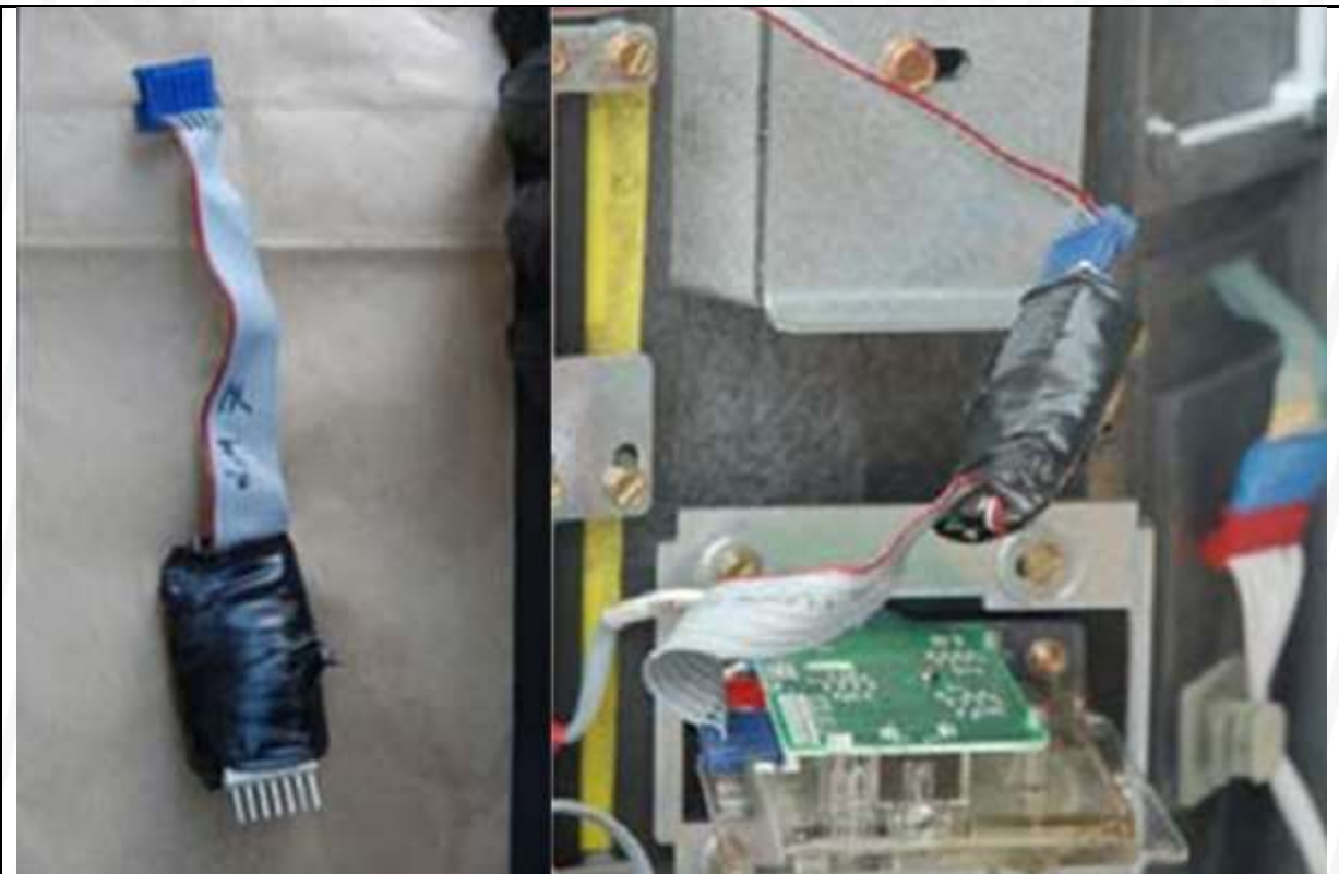
Example of internal fraud that connects directly to the card reader
