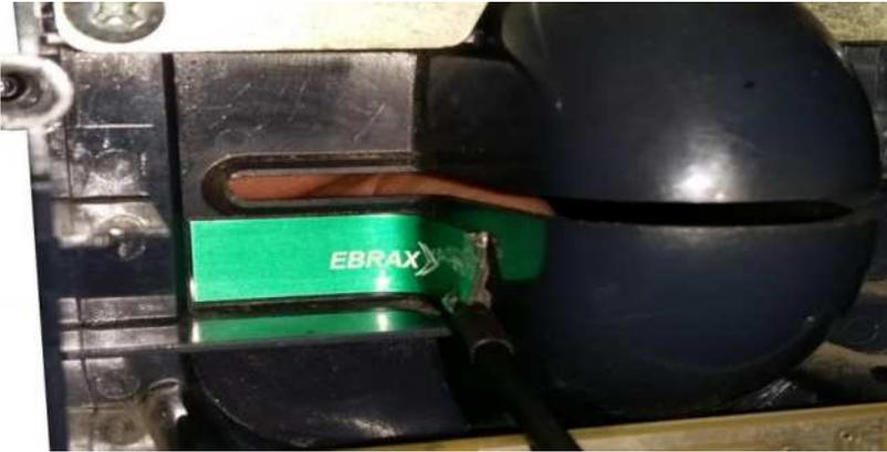
Figure 29. Antenna installed inside the card reader bezel
