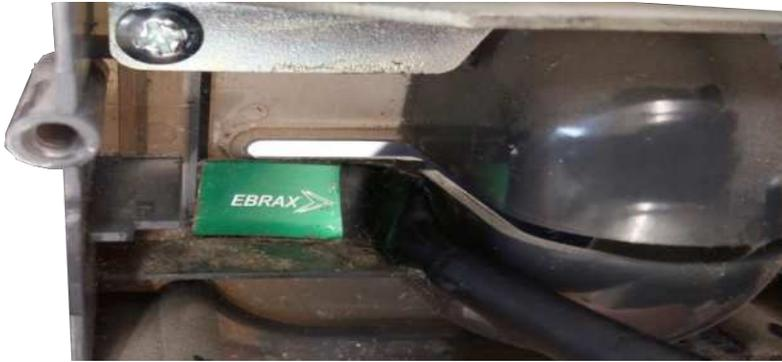
Figure 53. Antenna area with accumulated dust
