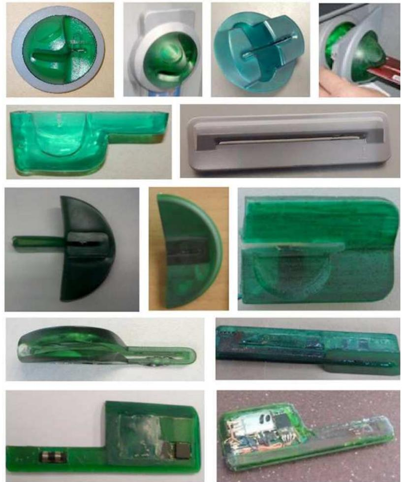
Figure 16. Example of overlay skimmers
