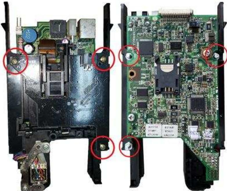
Figure 45. Screw tighten
