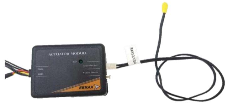
Figure 36. Transducer connection
