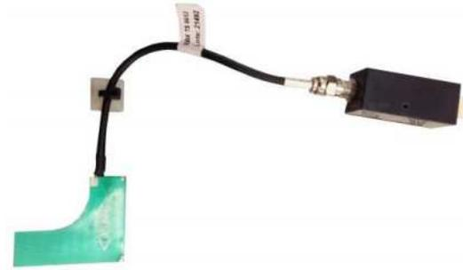
Figure 51. Correct example of antenna cable installation
