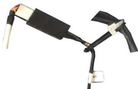
Figure 50. Excessively tight antenna cable
