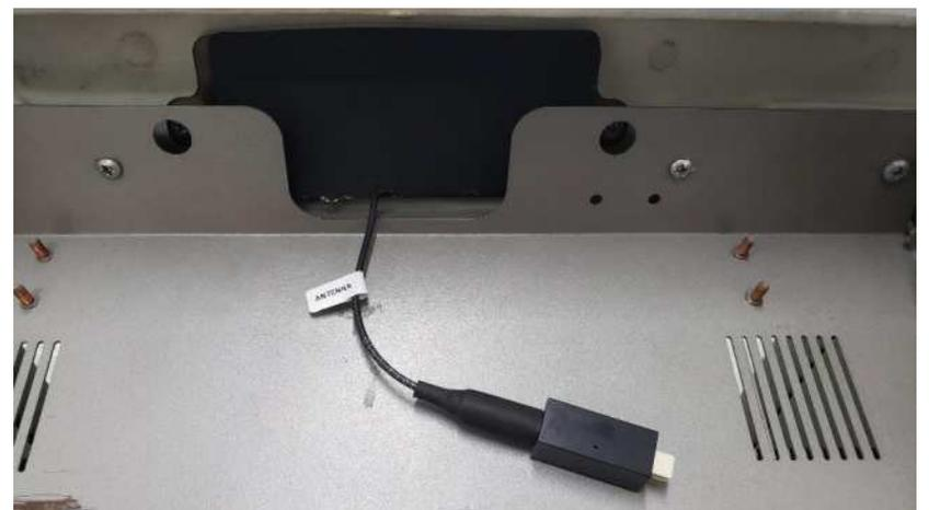
Figure 38. Example of correct sensor installation
