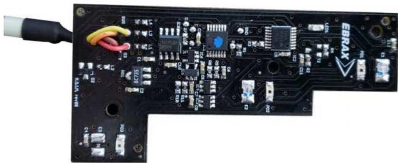
Figure 46. Custom sensor for motorized card reader
