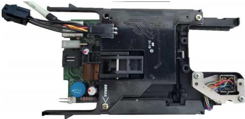
Figure 23. Deep insert sensor installed in the card reader
