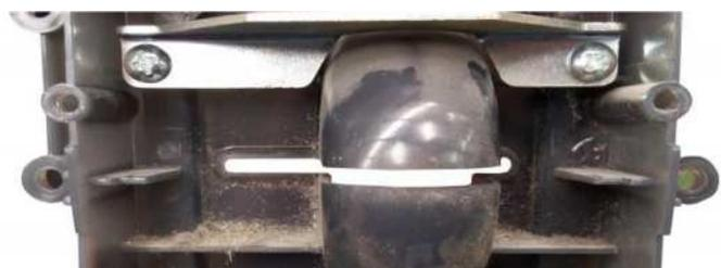
Figure 28. Installation surface needing cleaning
