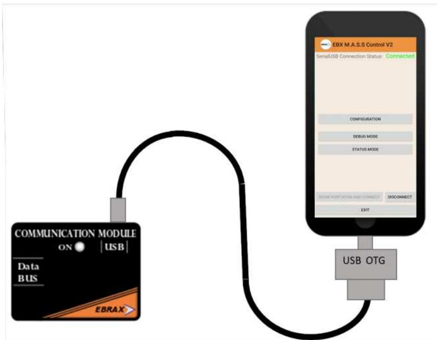
Figure 65. USB-OTG connection example
