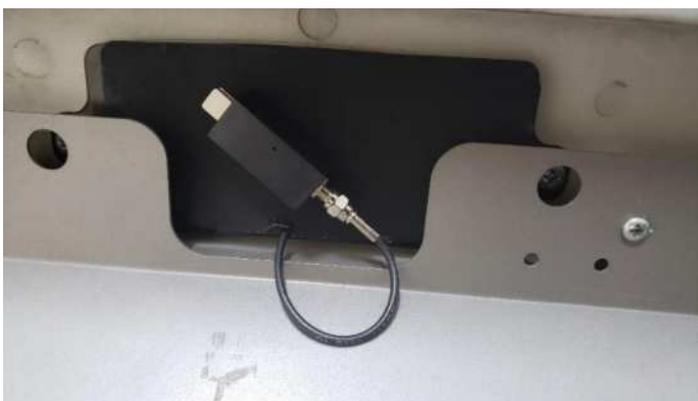
Figure 40. Overlay Sensor installed over the Antenna
