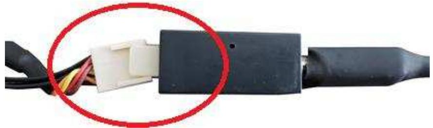
Figure 56. Wrongly disconnected cable
