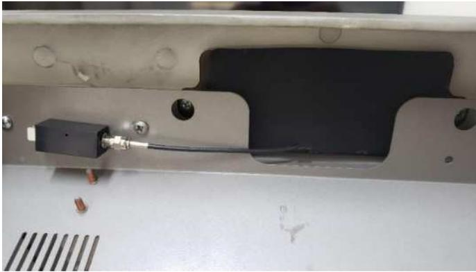
Figure 39. Antenna Cable too tight
