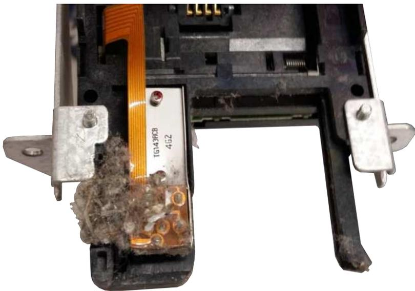
Figure 54. Card read with accumulated dust
