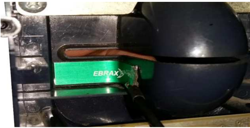
Figure 4 Antenna installation example
