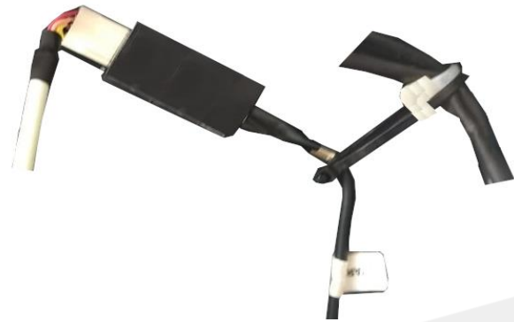
Figure 10 Incorrect Installation Example
