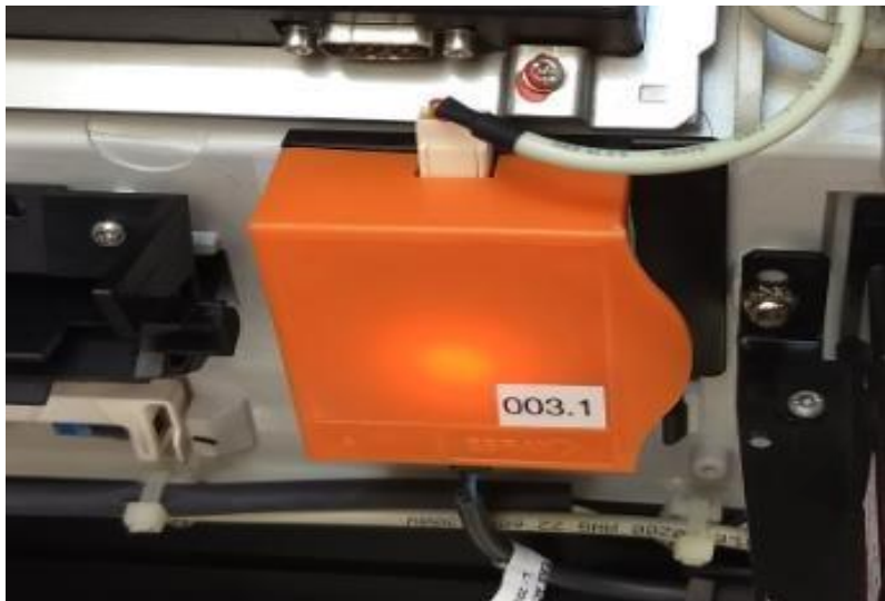
Figure 7 Installation of the Concentrator Unit
